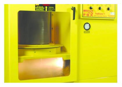
Soot and ash build up in a diesel particulate filter with time. After awhile, a DPF must be removed from the exhaust line and mechanically cleaned, as repeated regenerations will not be enough to address the ash buildup.
